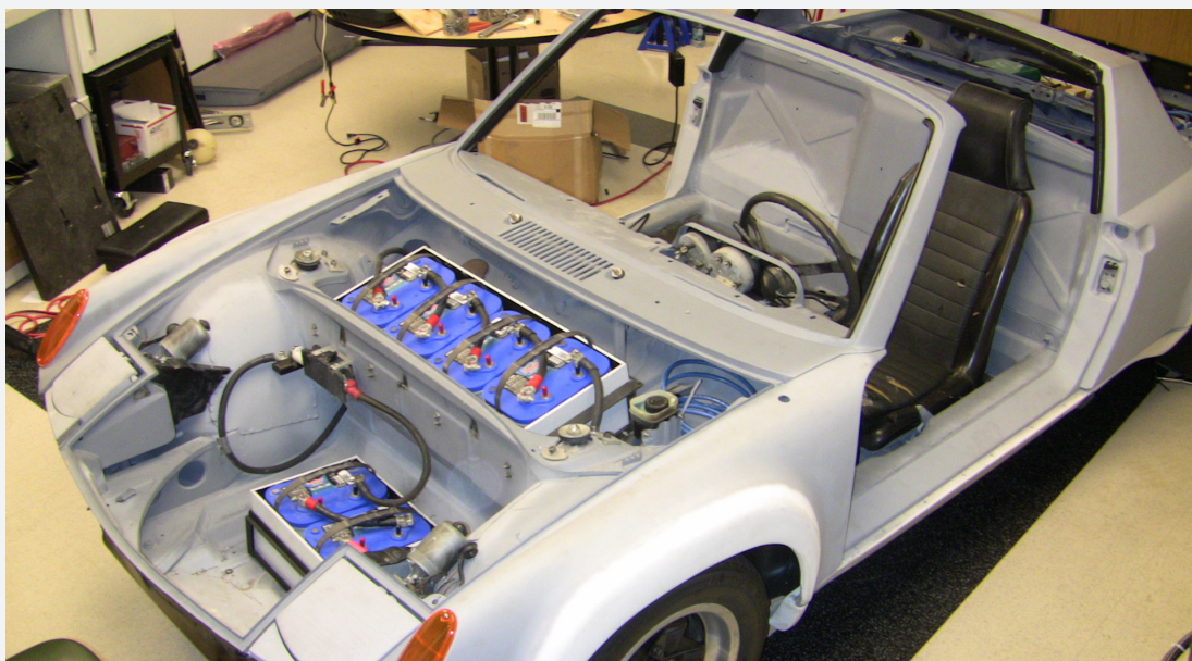
A group of engineering students turned an eBay purchase into an electric car, shown here in the basement of the Tucker Technology Center. The car has the body of a 1974 Porsche 914 Targa and is powered by a dozen 12-volt lead-acid batteries.
