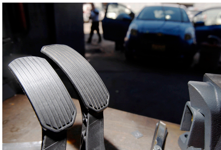
The gas pedal fix for recalled Toyota cars involves, among other things, shaving down the length of the pedal itself, as shown in the pedal on the left.
